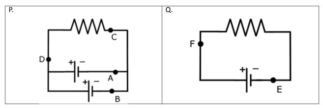
9. A flashlight manufacturer wants to design a flashlight for use in emergency kits. The flashlight should last as long as possible. His engineers come up with the designs shown below. Compare the currents they will draw from each battery and order them in sequence from the one that exhausts the batteries first (the hungriest circuit) to the one that makes the batteries last the longest (the least hungry circuit).
